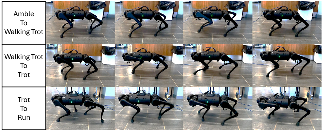
Figure 4.9: Snapshots of the gait transitions achieved through the bio-inspired gait transition method's hardware deployment.
